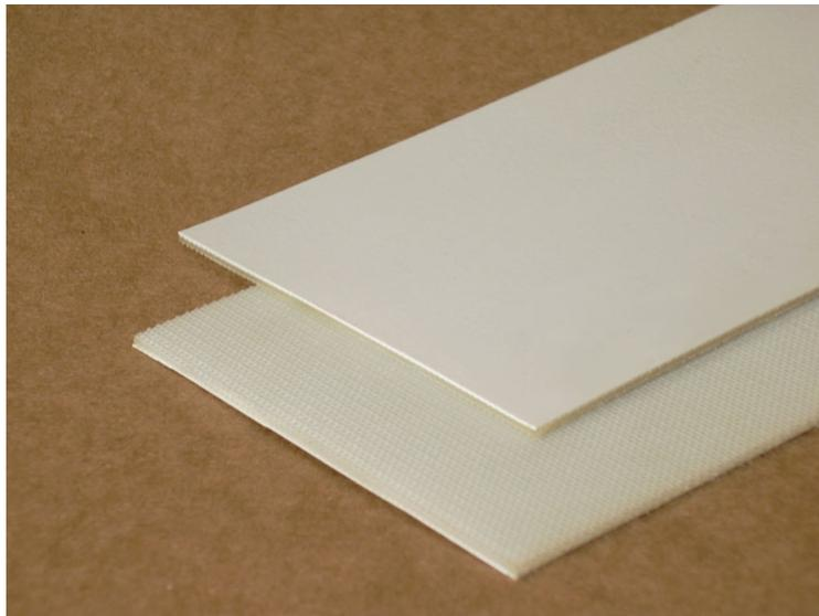
**Features:** This belt is a lightweight 2 ply monofilament construction that will negotiate small pulleys. The urethane compound is oil, animal fat and grease resistant. It is easy to clean and will lay flat. Refer to the chemical resistance chart when choosing a cleaning solution.
